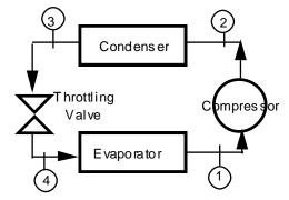
The state points for the cycle are shown on the diagram. For the ideal cycle there is no pressure drop or work in a heat transfer device so  $P_1 = P_4 = 0.12$  MPa and  $P_2 = P_3 = 0.7$  MPa. The compressor is assumed to be isentropic so  $s_2 = s_1$ . State 1 is a saturated vapor and state 3 is a saturated liquid.
