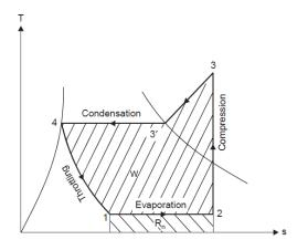
Given:  $h_2 = 183.19 \text{ kJ/kg}; h_3 = 209.41 \text{ kJ/kg};$
