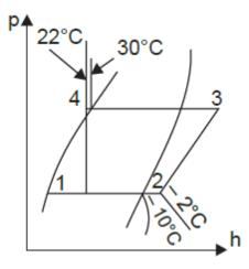
(i) Mass of a refrigerant circulated per minute: The values of specific enthalpies and specific volume read from p-h diagram are as under:
