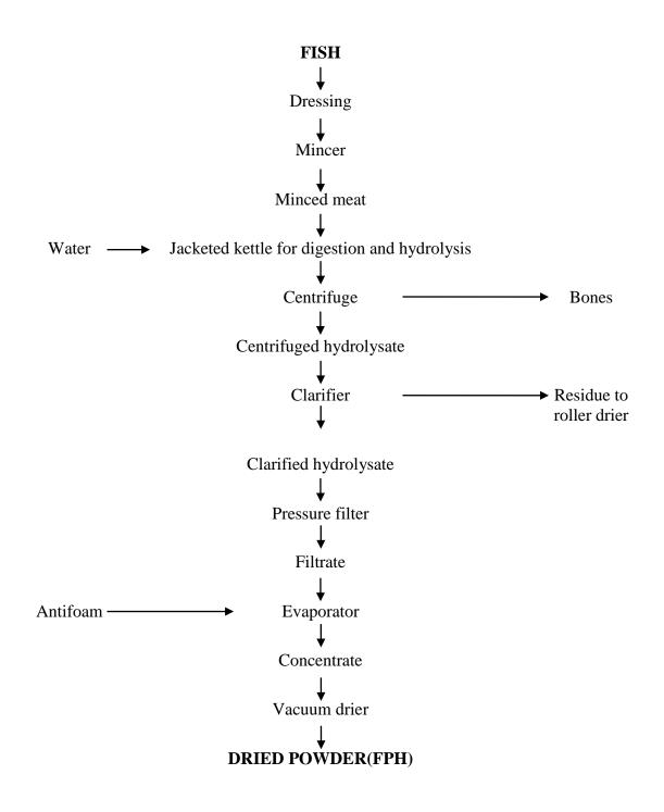
**Fig. 1.** Essential processing steps for the production of fish protein hydrolysate (FPH) *Source:* Sen 2005
