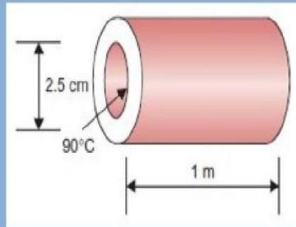
{Hint: Find the Reynold's number value to know fluid characteristic and then apply appropriate correlation to calculate heat transfer coefficient}
