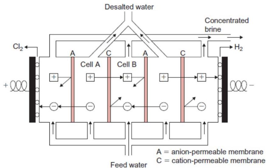
**Figure 4:** Desalting of water with an electro dialysis system.
