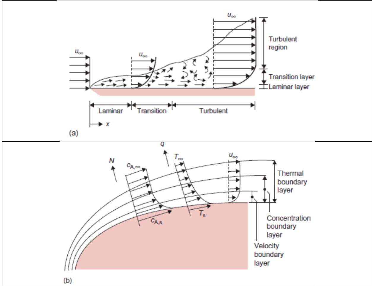
**Figure 1:** (a) The development of a boundary layer on a flat plate. (b) The development of the thermal, concentration, and velocity boundary layers on a surface.
