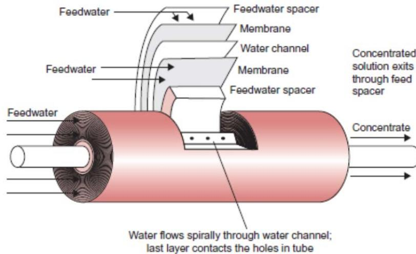
**Fig. 9:** A spiral-wound membrane system with a cross-sectional view showing the water flow patterns.
