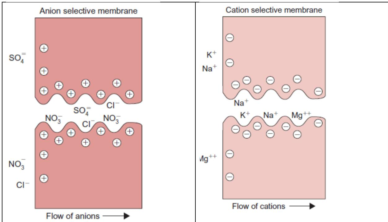
**Figure 3:** The movement of ions in ionselective membranes.
