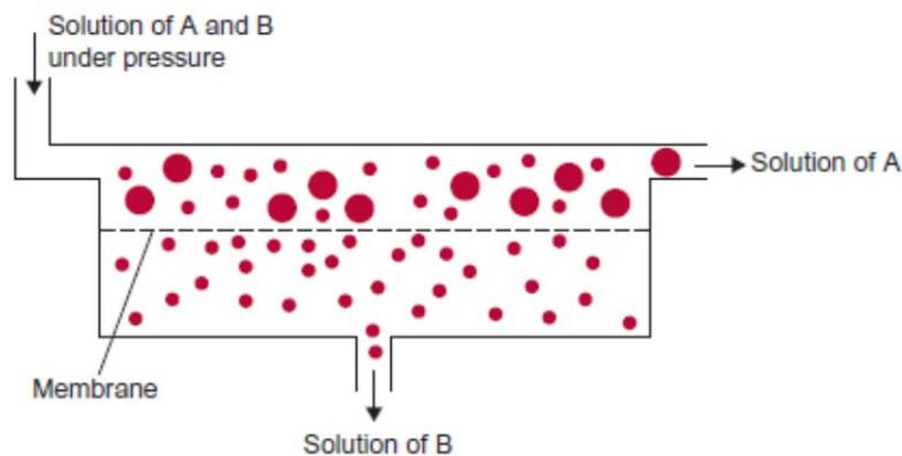
**Figure 6:** Separation process in a pressure-driven membrane system
