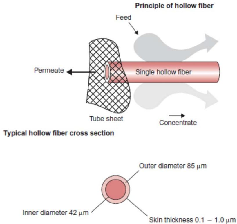
**Figure 10:** A hollow-fiber membrane system
