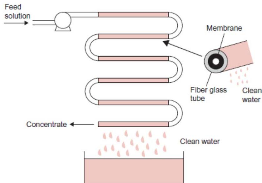
**Fig. 8:** A tubular membrane system.
