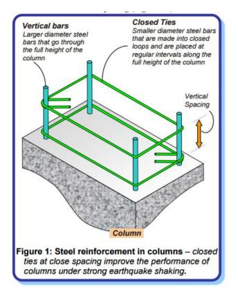
Columns can sustain two types of damage, namely axial-flexural (or combined compression-bending) failure and shear failure. Shear damage is brittle and must be avoided in columns by providing transverse ties at close spacing.
