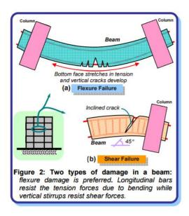
(b) Shear Failure:
