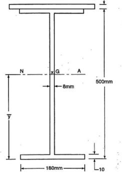
$\bar{y}$  = Moment of area about bottom fibre/total area of compound section =(240x12x506+180x10x495+180x10x5+480x8x250)/
