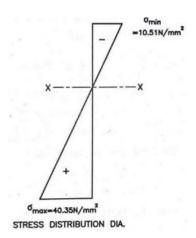
4. A rectangular column is 100 mm wide and 60 mm thick. It carries a load of 100KN at an eccentricity of 10mm in a plane bisecting the thickness. Find the maximum and minimum intensities of stress in the section.
