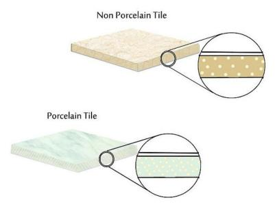
pattern of the finished tile; although an assortment of tile dyes are used for coloring. They are used in both wall tile and floor tile applications and are softer and easier to cut than porcelain. These non-porcelain ceramic tiles are usually suitable for very light to moderate traffic as they are more prone to wear and chipping than porcelain tiles.
