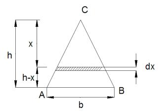
Consider an elementary strip PQ located at a distance of 'x' from the apex 'C'.
