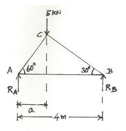
Length of the member  $AC = 4 \times \sin 30^{\circ} = 2m$ Therefore,  $a = AC \times \cos 60^{\circ} = 1m$   $\underline{SV = 0}$   $R_A + R_B - 5 = 0$   $R_A + R_B = 5 - - - - (1)$   $\underline{SM_A = 0}$   $5 \times a - R_B \times 4 = 0$   $R_B = 1.25 \text{ kN}$ From (1),  $R_A = 3.75 \text{ kN}$
